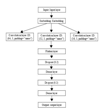
Figure 3 The layer architecture of the proposed CNN model.
